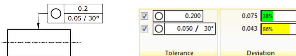
For the evaluation of the roundness or cylindricity, a Chebyshev compensation element is calculated, independent from how the tolerated element has been measured. This ensures the standardized evaluation according to ISO 1101.
