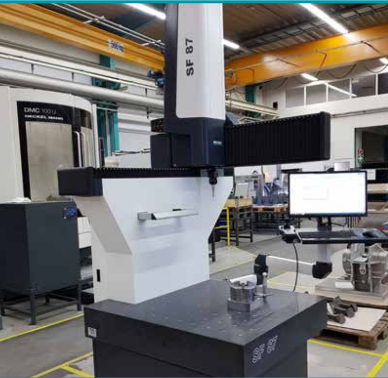
Figure 2: A modern production measuring machine is optimized to a minimum footprint (here just 2.3 m 2 ) and ergonomically designed for easy operation.
