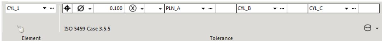
You specify the tolerance zone, the tolerance value, the calculation type and the reference system in the same way as you know it from the construction drawing.
